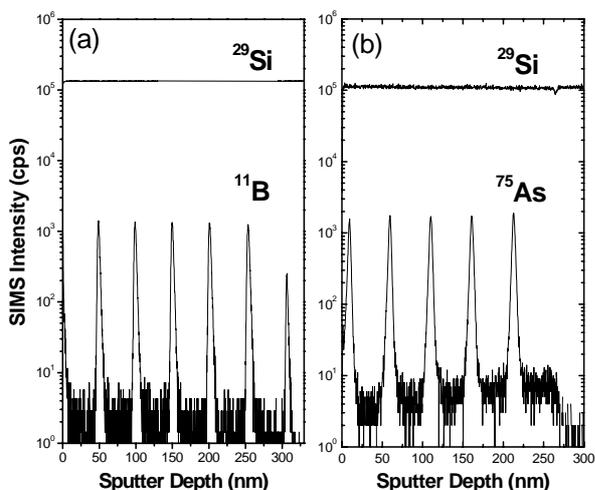
Fig. 2. SIMS depth profiles of typical multiple delta-layers with (a) B and (b) As-doped Si marker layers.
