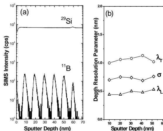
Fig. 4. SIMS depth profiles of a B-doped Si multiple delta-layer (a) and depth resolution parameters (b).
