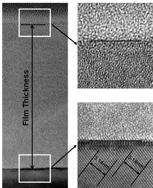
Fig. 1. Certification method of film thickness by HR-TEM based on Si lattice constant.
