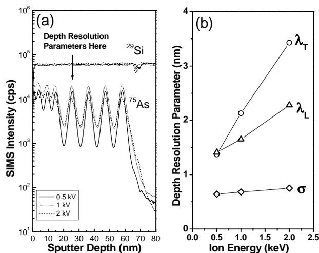
Fig. 3. SIMS depth profiles of As-doped Si multiple delta-layer with various ion energies (a) and depth resolution parameters (b).
