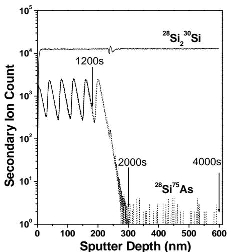
Figure 5. Overlay of 3 SIMS depth profiles of a GaAs-doped Si multiple delta-layer with different crater depths.
